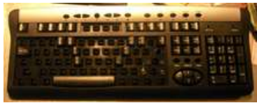
104-key USB keyboard adapted into a chording keyboard
